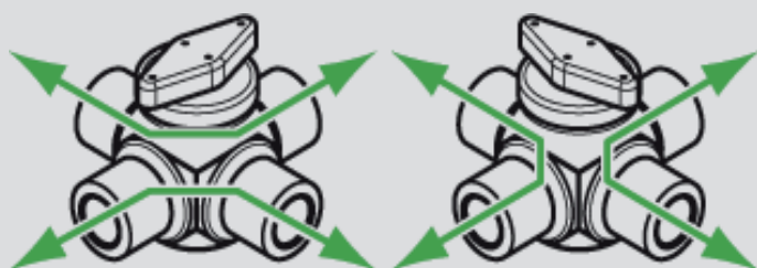
6L744F - 4-way with double L bore
