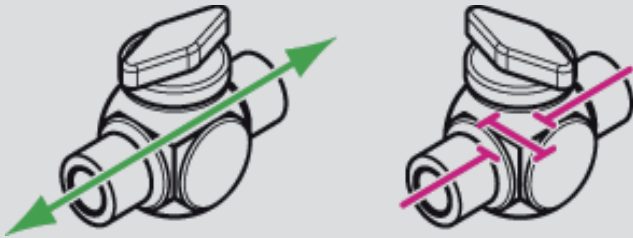
6L701 - 2-way with through bore
